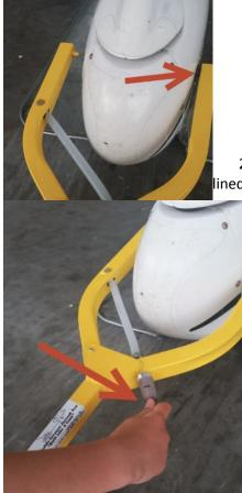
2. Using the crank, tighten the tow bar while keeping it ined up with the passenger-side lug on the nose wheel.
