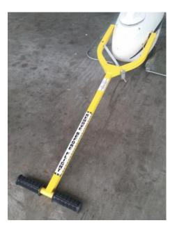
To remove the tow bar, reverse the process, again being careful not to scratch the nose wheel pant as you remove the tow bar.
