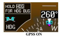
When GPSS is selected on the PFD, the heading bug on the HSI changes to a hollow outline and a crossed-out heading bug appears in the PFD Knob Mode Indicator, indicating that the autopilot is not coupled to the heading bug. The bug is still controllable and may still be used by the pilot for reference.
